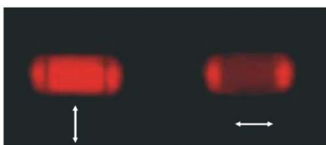
Fig. 7 Polarised fluorescence microscopic pictures of a 2.5 \mu\text{m} long \text{Ox}^+ -loaded zeolite L crystal after excitation at 545\text{--}580 \text{ nm} (cut-off 605 \text{ nm} ). The arrows indicate the transmission direction of the polariser.
